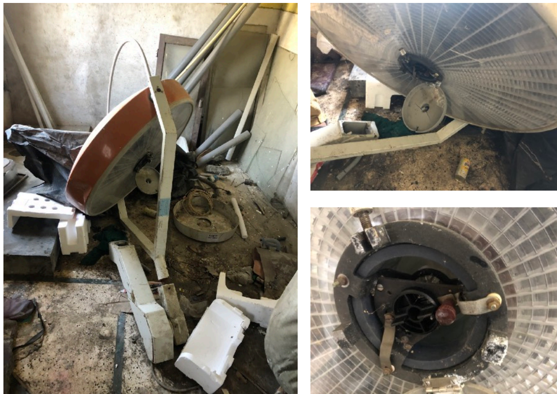
Figure 3: Left: The donated coupled OT-light at JHCRC is disassembled and stored at a store room covered with moulds. Top Right and Bottom Right: Close up of the OT-light.
